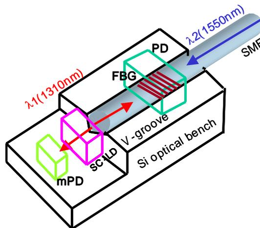
Fig. [6] Schematic configuration of fiber in-line transceiver for WDM PON system
